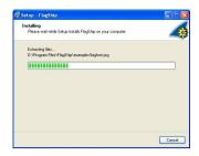
Now, the setup wizard installs FlagShip in the selected directory (usually in C:\FlagShip7 or C:\Frogram Files\FlagShip7). It additionally creates or checks ...\borland\bcc55\bin\\*.cfg files for BCC32 and creates batch file named *FlagShip\_console.bat* in the installation directory. This batch file is assigned to the "FlagShip7 BCC Console" icon on your desktop.
